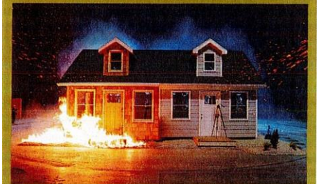
Figure 2b Embers impacting a building: left side with combustible (wood) and the right with noncombustible (rock) mulch.
